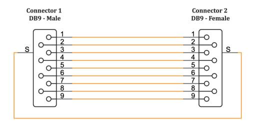
Each pin of the DB9 connector is electrically connected to a single row of the prototyping area and the corresponding pin on the opposite connector. The pads of the prototyping area have a standard 0.1" pitch.
