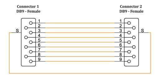
Each pin of the DB9 connector is electrically connected to a single row of the prototyping area and the corresponding pin on the opposite connector. The pads of the prototyping area have a standard 0.1" pitch.
